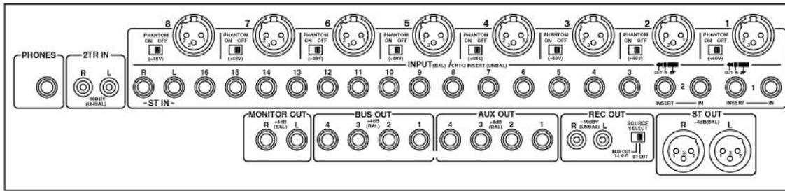
Monitoring to amplifier and speakers is from the MONITOR OUT (1/4" TRS) connections
