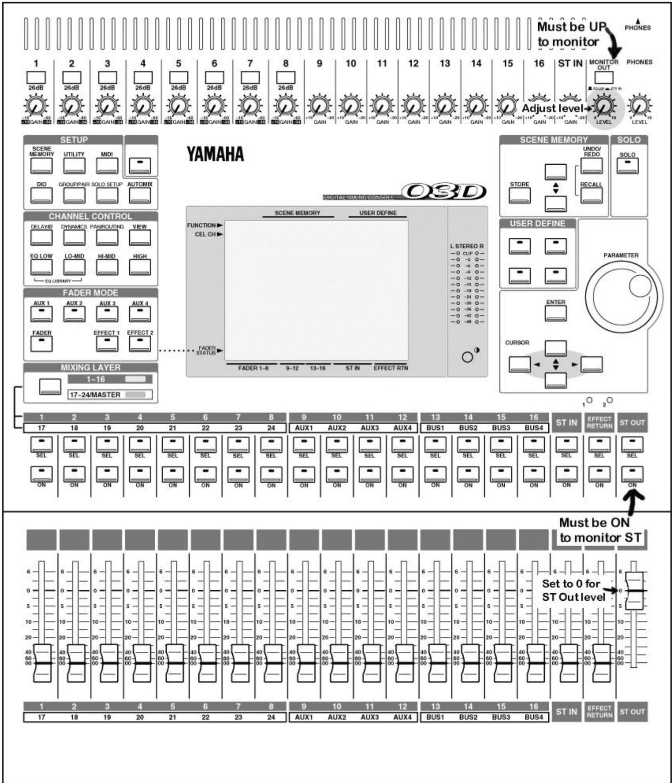
Note: The 03D ST OUT is used for monitoring (VU meters active) and Program Output. Ensure the ST fader is up to 0 level, the ST ON lamp is illuminated, and the MONITOR OUT button is in the UP position.
