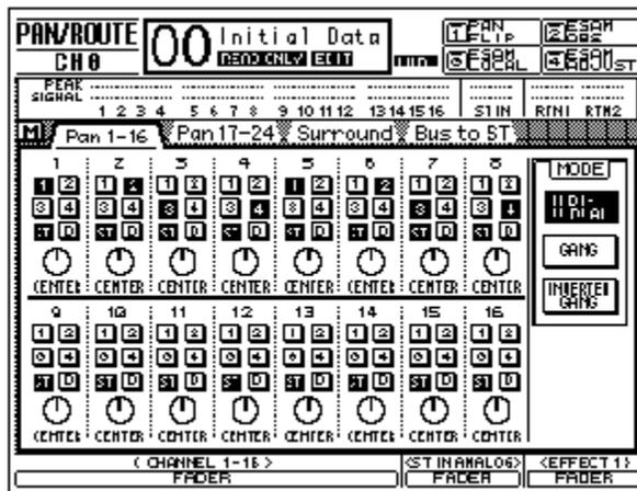
The BUS Outputs (1-4) are fed to the RECORD device for recording (or AES Out if the YGADI option is installed) and the MONITOR OUT connected to amplifier and speakers. The ST OUT is the signal that is monitored on the MONITOR OUT (when set in [Bus to ST] to OFF {not highlighted}), allowing preview monitoring to be controlled via the 03D mixer. The MONITOR OUT has a volume control knob for convenient speaker volume adjustment.
