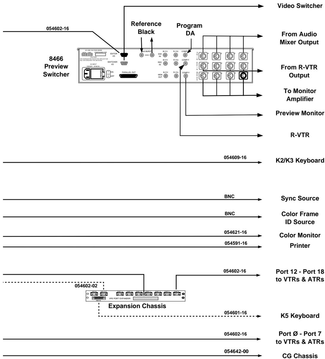
Figure E-2. Example of System Interconnection With an 8466 Preview Switcher
