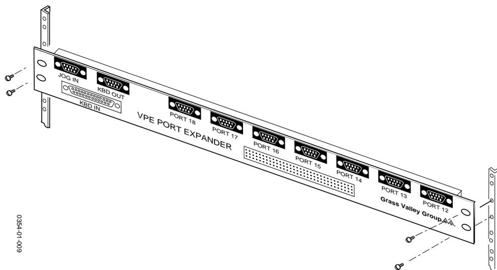
Figure 3-5. Expansion Chassis Installation
