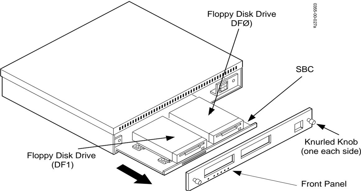
Figure 3-3. Removing the SBC
