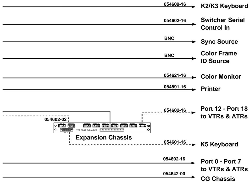
Figure E-1. Example of System Interconnection Without an 8466 Preview Switcher
