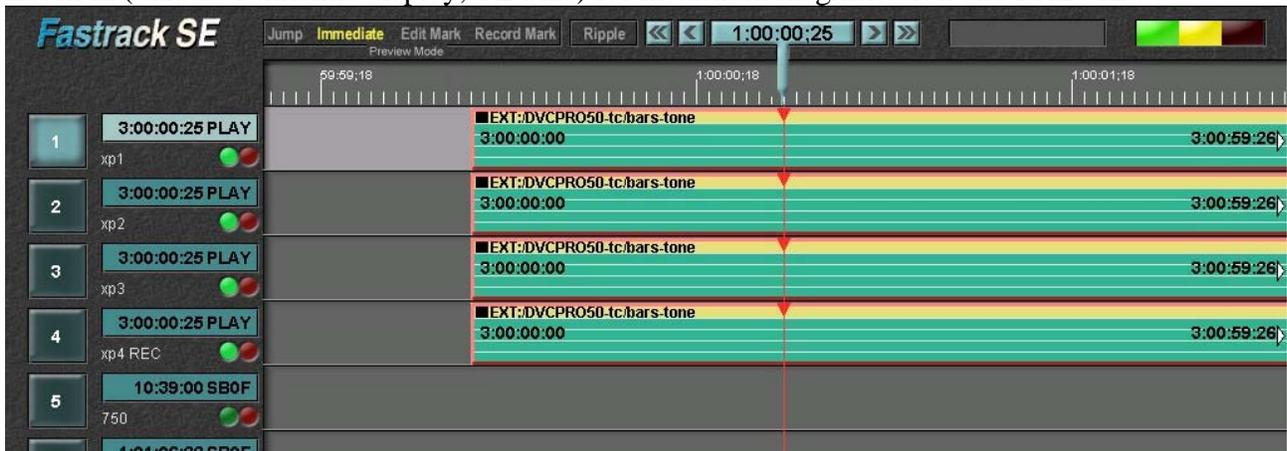
The image above shows correct CPI positions (Current Position Indicator; the downward pointing red triangle on the video line of each event) for each track precisely synchronized at the red vertical line representing the current timeline time (under the CTI; Current Timeline Indicator which reads 1:00:00;25). The CPI shows the current relative position on the event, representing that position on the event by the "play head" (timecode in the STATUS area (3:00:00;25) is the current position.
