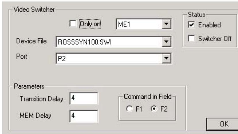
*For the Ross Synergy 100 shown above, the **Transition Delay** is set at **4** and the **Command in Field** is set to **F2** for precisely switched source timing*
