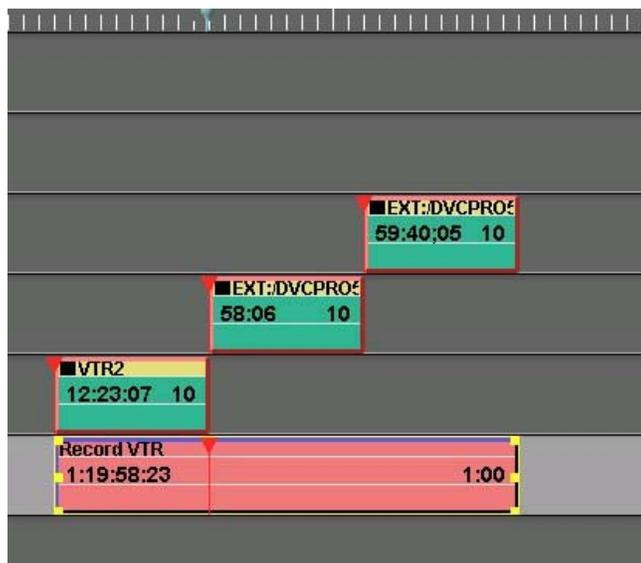
If switcher timing is correct, you will SEE the switch to the second event at the first field of the **tenth** frame into the recorded edit, and between the second and third events at the **twentieth** frame into the recorded edit (shown below)
