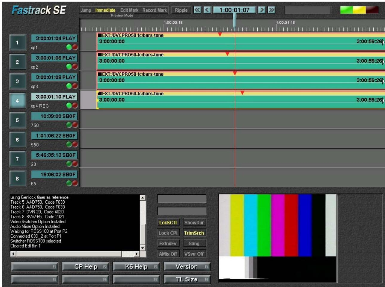
If the CPI for any channel is 'offset' from the CTI during a preview (as Track 1, 2, and 4 above), then adjust that individual track's Frames Offset by highlighting the track and pressing [INIT]. Each Profile should have the same Frames Offset on all channels (unless going through a different video path into the video switcher).
