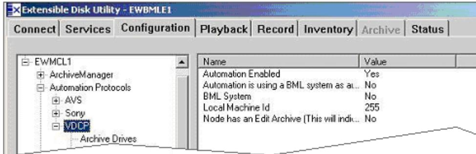
3. Select the VDCP **Communication Ports** that are to be used. (Ex: COM5, COM6, COM7) and enable **Serial Communication**.
