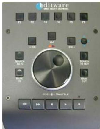
*The outer ring of the knob is for variable speed and shuttle (the middle button above the knob selects Var (lit) or Shuttle (unlit)). The inner knob is for frame by frame jogging.*
